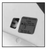
Your vehicle is equipped with rear door security locks that help prevent passengers from opening the rear doors on your vehicle from the inside.
